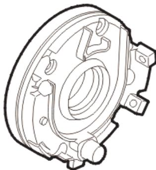
The oil pump pumps oil from the oil pan via channels in the intermediate section and cylinder block into the cylinder head and onwards in the system. The oil pump is on the end of the crankshaft. The crankshaft runs through the oil pump.
