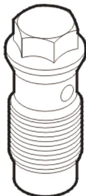
The piston cooling valve is manufactured in steel with a hardened piston, a spring and a spring stop. A copper washer ensures that oil does not leak onto the cylinder block.
