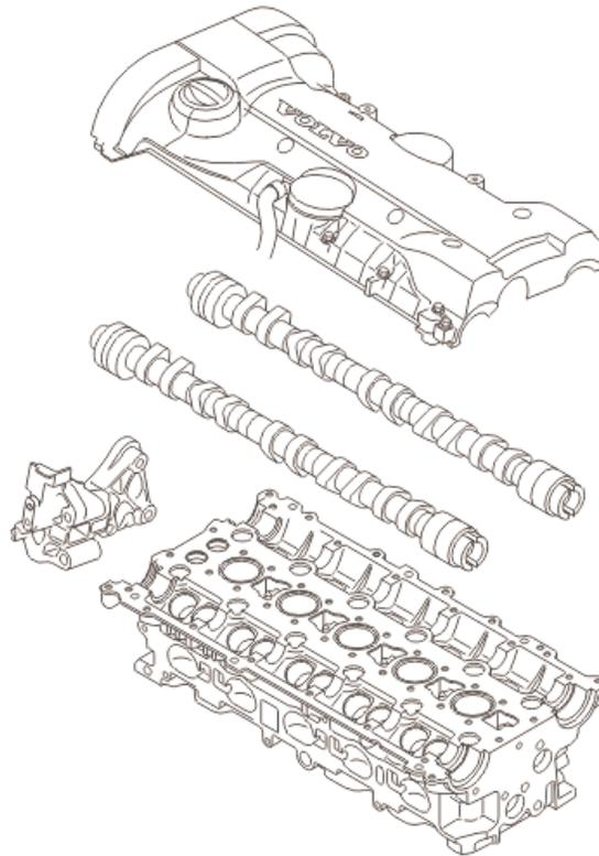
The entire engine is manufactured in aluminum. The engine block is divided up into five sections. The cylinder head consists of two sections and the cylinder block of three sections. The seal between the cylinder head and cylinder block is a conventional cylinder head gasket. The seal between the other gasket faces is a liquid gasket.
