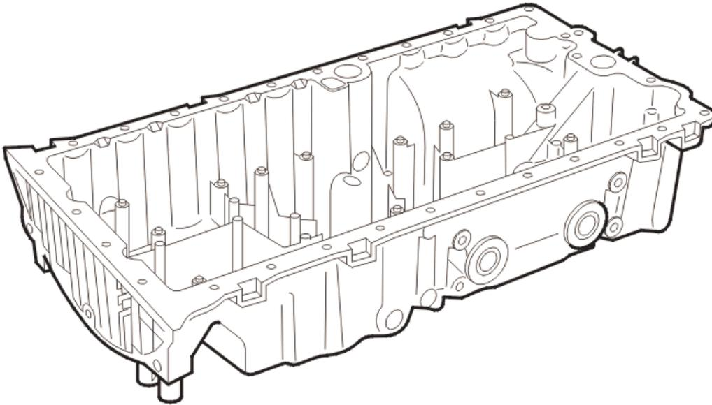
The oil pan is made of die cast aluminum with baffles. This is so that the oil does not splash excessively. It is secured in the cylinder block with a liquid LOCTITE gasket, which ensures the seal between the cylinder block and oil pan.
