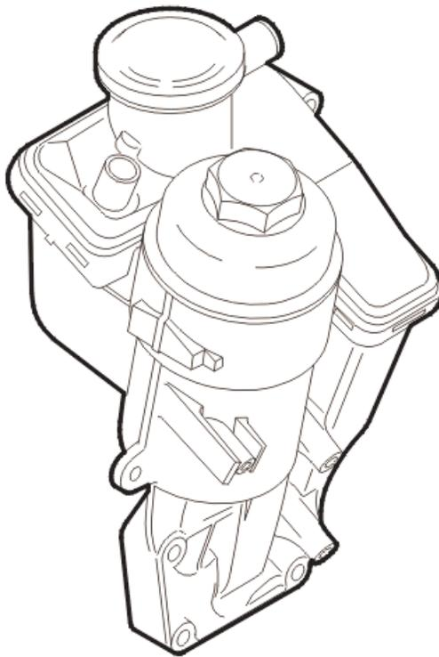
The oil filter holder is made of die cast aluminum. It is on the cold side of the engine. The oil filter cover is plastic. There is a by-pass valve in the cover. An O-ring in the cover ensures that it is
