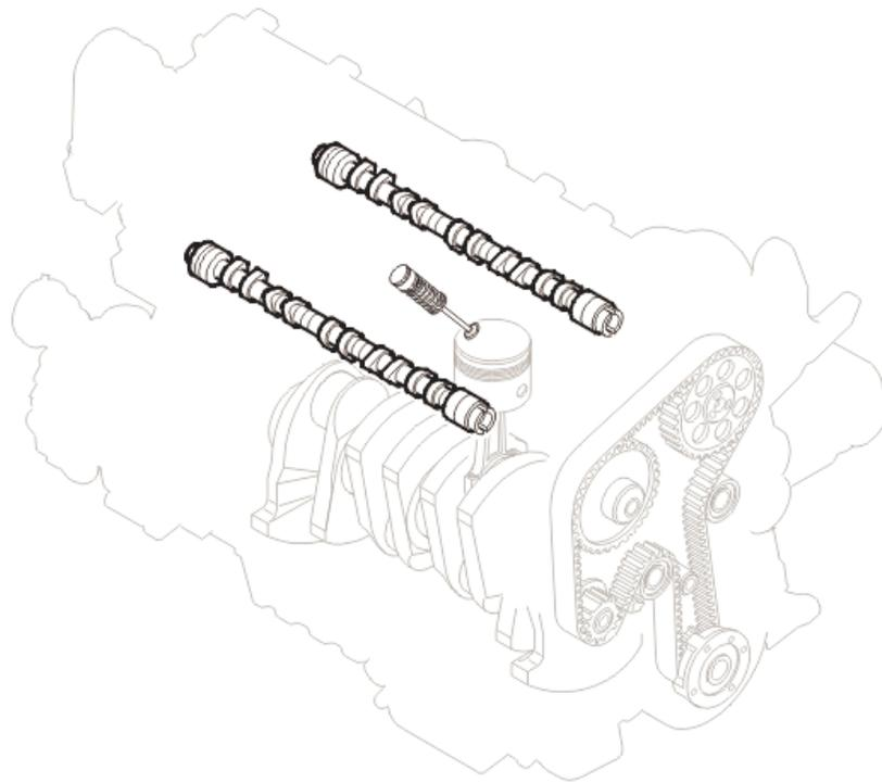
The camshafts are cast iron. The cam lobes which press against the valve lifters are harder to tolerate the contact pressure. The valve lifters are steel and mechanical, not hydraulic.
