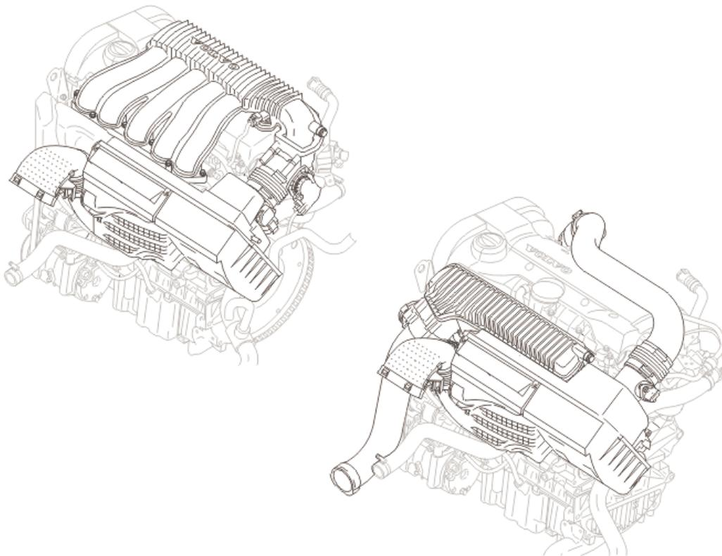
The intake system is divided into two sections, the upper and lower intake manifolds. The upper intake manifold is made of plastic for naturally aspirated and turbocharged engines. The lower intake manifold is aluminum for both types of
