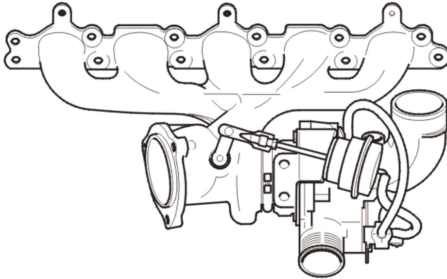
The integrated manifold and turbine housing are made of austenite forged steel to tolerate exhaust temperatures up to 1050 °C.
