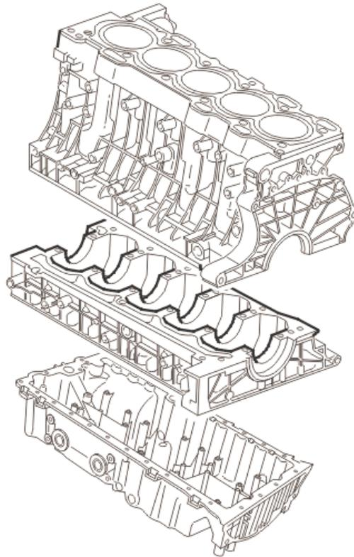
The engine block is divided into three sections, the cylinder block, intermediate section and oil pan. The mating flange between the cylinder block and intermediate section is in the center line of the crankshaft.
