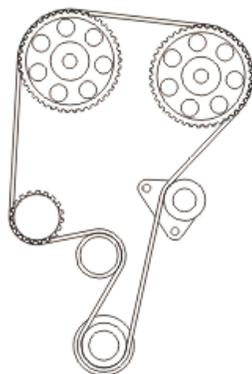
The tensioner consists of a spring and a friction element. The friction element provides the required damping to absorb small oscillations and speed variations. The spring ensures correct belt tension, irrespective of wear and temperature. The belts are made of cord reinforced rubber.
